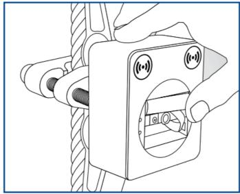
IN A SAFE AREA ONLY, remove the side cover of the BOLT using a flat blade screwdriver. Fit batteries and refit cover.
