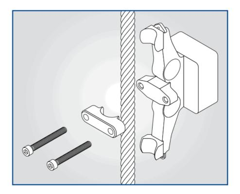
Remove the two M10 bolts of the device place the device under the rope being measured attach the top clamp and tighten the bolts.
