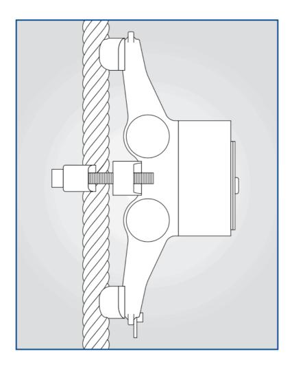
Make sure the bolts are torqued up equally, the torque rating is provided on the calibration certificate. **Note:** It is important that the two bolts are tightened equally, if not it could show incorrect readings
