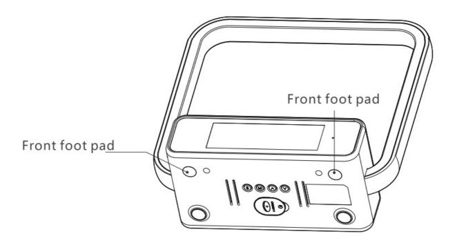
Screen brightness adjustment Tap the snooze button(2 front foot pads) to adjust the brightness of the screen, Highlight — Medium — Low — Off
