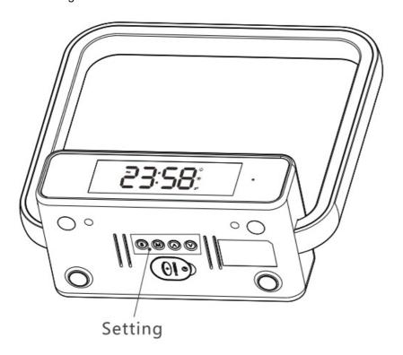
Short press "S" to switch 12/24 hours, press 2 seconds to enter set time mode, the sequence is: hour/ minute, the set item blinks, press "A" or "V" to turn up/down to set time. Long press for two seconds to quickly adjust, no hope ration 5 seconds automatically exit.
