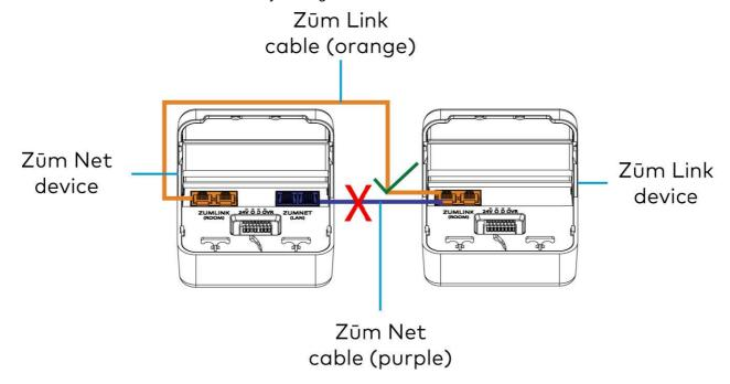
Use orange CBL-CAT5E-ZUMLINK-P cables (sold separately) to wire in- room Zūm wired devices, such as load controllers, to the ZUMLINK-KP.
