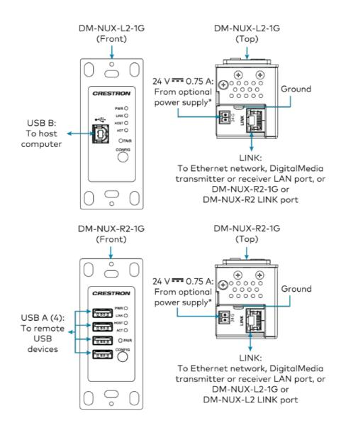
Connection to a 24VDC power supply is not required when PoE is used to power the USB extender or when the DM-NUX-L2-1G is connected to the Host device.
