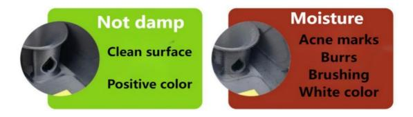
\*The model shown is a display of a common filament material under moisture.
