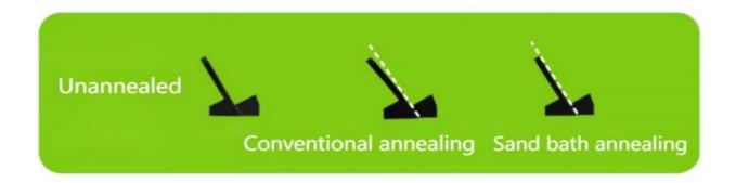
\*It is important to note that the annealing process is usually accompanied by shrinkage and deformation of the model, so you need to be careful in choosing whether or not to anneal the model.
