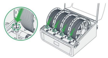
Loading filament: Put the filament into the CFS, align the filament head with the Teflon tube of corresponding silo, push it in gently, and let go after feeling the pulling force. The filament will be automatically loaded.
