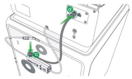
4. Connect the CFS to the printer using the 485 communication wire: This cable has 6-pin straight connectors on both ends with no specific orientation.
