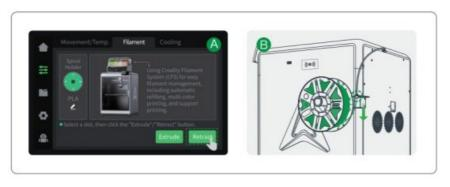
During extruding, you can observe whether there is filament flowing out of the nozzle. If no flow-out is observed, you can gently push the filament toward the extruder at the Teflon tube behind the machine, and then click "Extrude" again.
