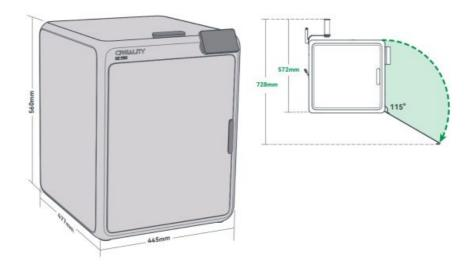
Overall machine dimensions ( $477 \times 445 \times 560$ ), including the top cover handle, front door handle, and foot pads.
