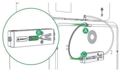
3. Connect CFS and buffer Creality 485 cable: Note that the elbow is inserted into the buffer position c, and the straight head is inserted into the CFS position d (either of the two 485 sockets of CFS).
