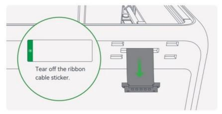
2. Connect the screen cable: Pay attention to the direction shown in the figure and press to connect.
