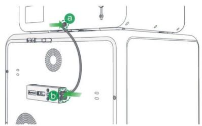
2. Connect the buffer to the printer following steps A, B, and C.
