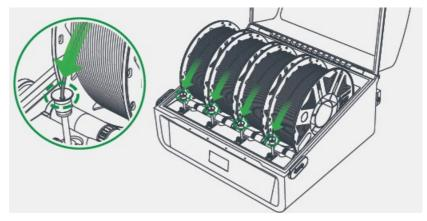
Loading filament: Put the filament into the CFS, align the filament head with the Teflon tube of the corresponding silo, push it in gently, and let go after feeling the pulling force. The filament will be automatically loaded.
