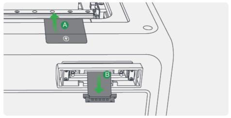
3. Connect the screen cable: Pay attention to the direction shown in the figure and press to connect;
