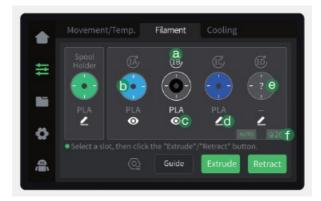
1. Introduction to the filament management interface: The filament management page is divided into two parts: the spool holder [left] and the CFS [right]. The code above the filament in the CFS, such as 1A, indicates the slot number;
