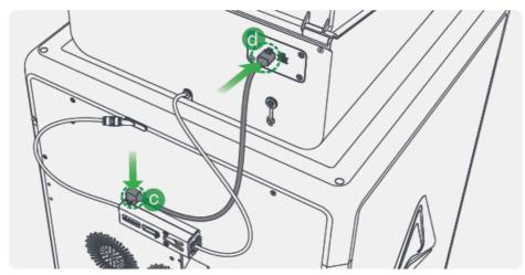
4. Connect CFS and K2 Plus Creality 485 cable: Both ends of this line are 6-pin straight heads, one end is inserted into the CFS position e, and the other end is inserted into the machine interface position f.
