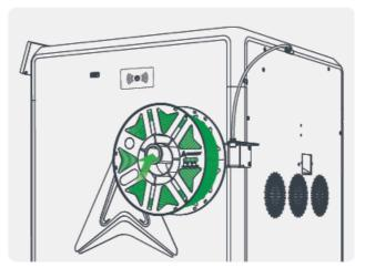
3. Thread the filaments into the Teflon tube and push gently until they cannot be pushed;
