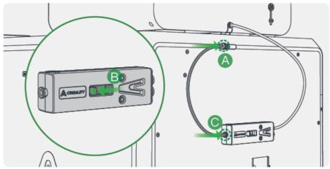
3. Connect CFS and buffer Creality 485 cable: Note that the elbow is inserted into the buffer position c, and the straight head is inserted into the CFS position d (either of the two 485 sockets of CFS);
