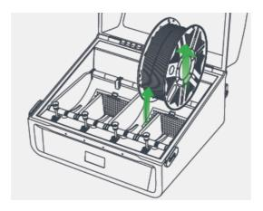
Unloading filament: First, make sure that the filament is not in the extruder, in this case, just pick up the filament and pull it out; if it is in the extruder, click the Retract button first, wait for the filament to return to the CFS, and then take out the filament.
