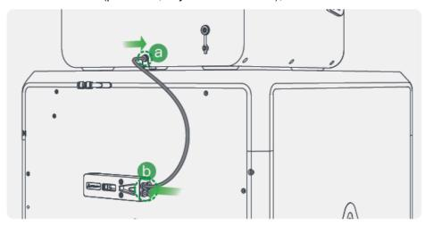
2. Connect the buffer and K2 Plus according to steps A, B, and C;
