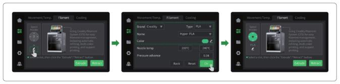
5. Extrude: Push the filament gently by hand, and click "Extrude" on the filament interface. The machine will automatically set the current filament temperature, and will automatically extrude the filament after the heating is completed;
