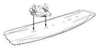
5. Put 2 pcs Hexa washers in place, one to the left and the other one to the right side of the Hexa footpad. Make sure the holes in the washer are aligned with the inserts on the board. Tighten 2 pcs screws slightly – left and right side of the Hexa footpad.
