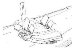
8. Take the Hexa II foots trap and open the Velcro. Thread the Velcro through the Quattro Stix. It is best to start on the Quattro Stix Long in the left side of the Hexa footpad right (inside of the foot). Then continue with threading the Velcro through the Quattro Stix Short on the same side.
