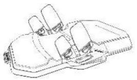
3. Adjust all Quattro Stix to the desired position. Make sure there is one empty position between Quatro Stix Short and Quattro Stix Long.
