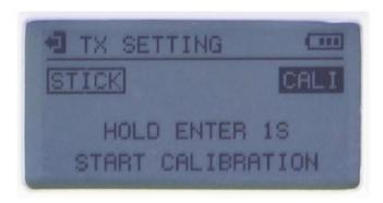
**7. Ver: 10602-LDA:** Select "SET", pop-up window prompt, "YES" to restore the factory, re-calibrate the neutral position of the remote bar after factory setting.
