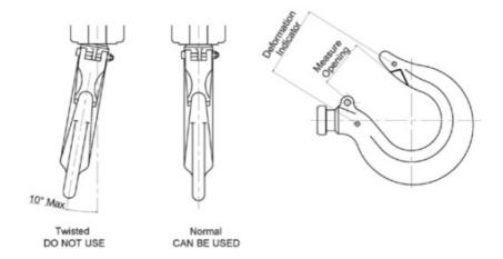
Any hook that is twisted or has excessive throat opening, indicated abuse or over loading of the unit. Other load sustaining components of the chain block should be inspected for damage.
