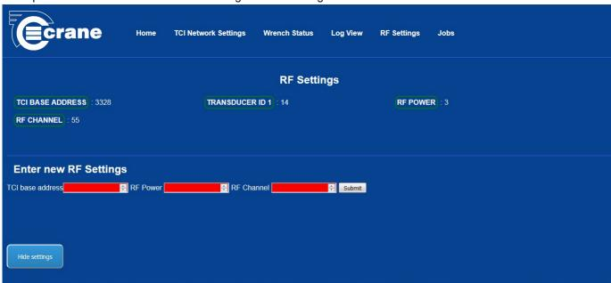
The TCI base address should be set between 1 and 65353. Each TCI should be given a unique base address so that WrenchStar Multi's Paired with a particular TCI will only communicate with that TCI and no other. The RF power typically gives the following ranges: 0 = 1m
