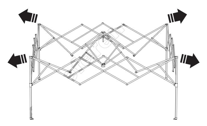
**STEP 1:**Gradually pull each leg/corner of the Gazebo Frame (A) outward to extend it fully on all sides. This gazebo can be opened by one person.
