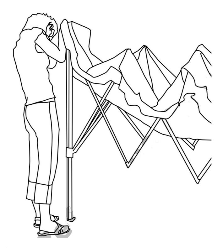
STEP 2: Place the Canopy (B) over crossbeams and ribs of Gazebo Frame (A). Connect all fasteners at the tops of each telescopic leg to the fasteners found on the inside-corners of the Canopy (B), and that the fastening straps are secured around the crossbeams.
