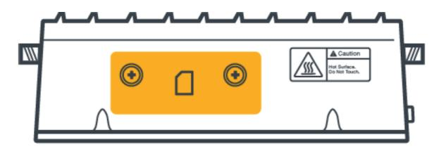
STEP 3: Insert an activated 4FF-sized SIM into the router
