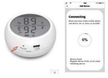
5. Under the automatic network configuration mode, press and hold the reset button with the Pin for 5 seconds to slow down flash of the indicator light as entering the manual network configuration mode. Choose the compatibility mode of APP and enter "WiFi password" according to the prompt and connect to network
