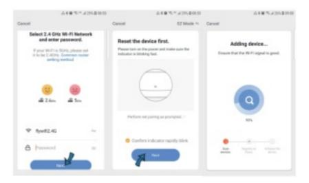
If your wifi router open both 2.4GHz and 5GHz with same name, please choose "AP Mode", enter the wifi password, hold the reset button for about 5 seconds till indicator blink slowly, connect your mobile to the device's hotspot: "SmartLife-XXXX", click to return to App interface, it will connect to wifi router automatically, the configuration complete. Push the back cover to close the battery compartment.
