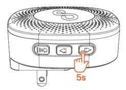
Press and hold down the Forward Button on the receiver for about 5s until it makes a "**Ding**" sound with LED light flashing, all the settings will be cleared.
