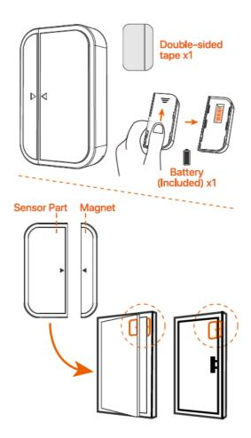
When the gap between the sensor part and the magnetic pole is greater than 0.4 inch (1cm), the sensor sends a signal to the receiver.
