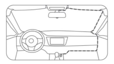
\*Please use a pry toll to hide the power line under the roof upholstery and seal the rubber ring along the A-pillar.
