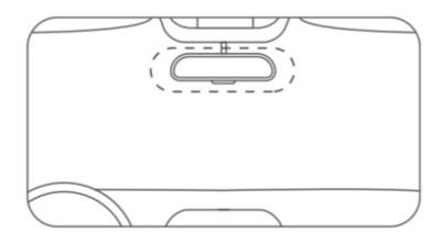
2. Insert the SD card into the connector with the contact side facing up, the SD card is installed until a (click) sound is heard.
