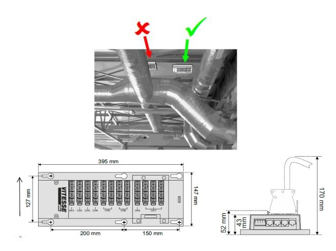
Install this way up: The unit MUST be installed this way up to ensure good lock of cable plug to socket.
