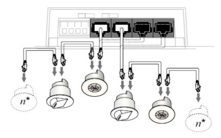
The power used by 1 microwave detector is the same as that used by 2 PIR detectors. These LCMs can supply power to a maximum of either 3 microwave detectors or 6 PIR detectors. You can connect combinations of
