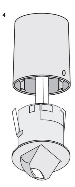
Secure detector to mounting box
