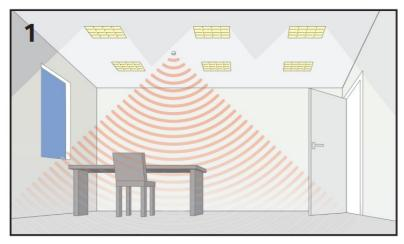
2. Vacate the room or remain very still and wait for the load to switch off (this should take less than 20 minutes).
