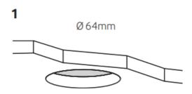
Cut a 64mm diameter hole in the ceiling.
