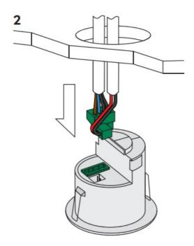
Wire in plug/s, using wiring diagram on page 2 as a guide. Connect the plug/s to the detector.
