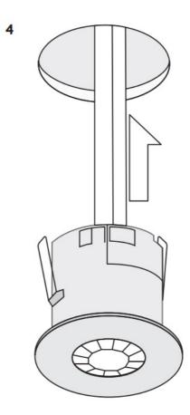
Bend the springs up and push detector through hole in ceiling. When fully inserted the springs snap back to hold the device in place.
