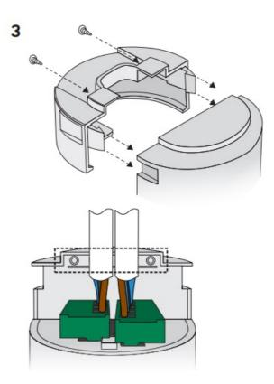
Continue tightening the screws until the clamp bar snaps out and is tightly engaged against the cable/s. The cable clamp must clamp the outer sheath only.
