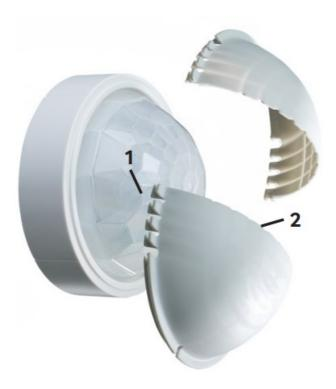
The detector includes two clip-on masking shields, enabling precise masking of the detection shape for aisles and corners as well as narrowing the detection diameter.
