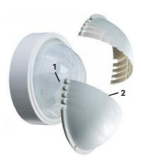
The detector includes two clip-on masking shields, enabling precise masking of the detection shape for aisles and corners as well as narrowing the detection diameter.
