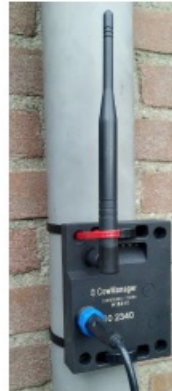
Example of using cable ties to mount the WIB2000 on a pole.
