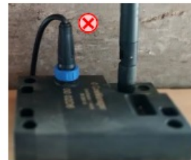
Avoid sharp bending of the USB cable.
