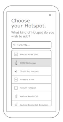
• Step 4: Following the App operation steps to reach below user interface, then press the BT button 5 seconds to turn on the gateway BT for pairing and then click "Scan for my Hotspot".
