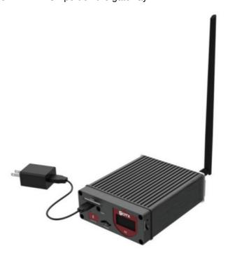
After the power connection, the LED would light up and turn green when it's ready for further configuration. IP address would show on the screen for Ethernet cable connect to WAN/Internet scenario. Click the BT button and the screen will display the Ethernet IP and device status.
