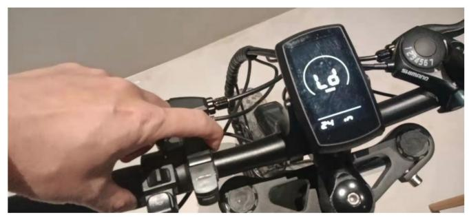
5. speed which can be added/subtracted through UP+/DOWN- keys
