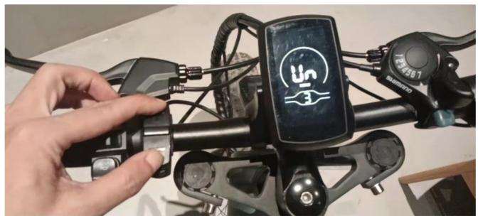
3. Press and hold the "-" and "i" key for more than 2 seconds at the same time to enter the wheel diameter setting interface.
