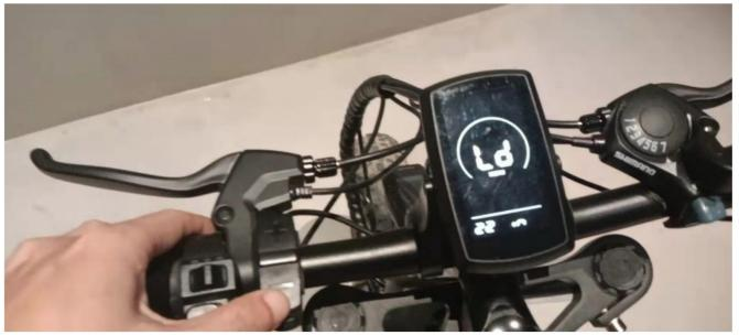
6. Press the "i" key for a long time to confirm and exit the setting state.
