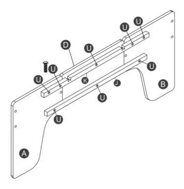
Align the A-B board and the L-I bar with the screw holes (as shown in the diagram), and tighten the U screw to secure the A-B-L-I components.
