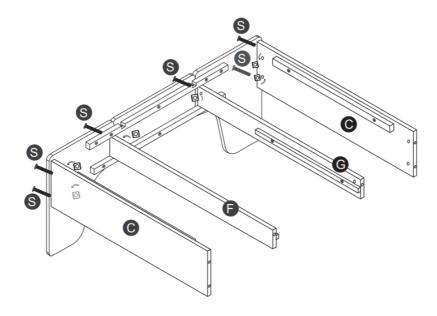
Secure the components from step 2 onto the components from step 3 using the S screw and nut (as shown in the diagram).
