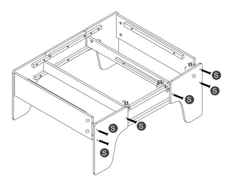
Install the H bar onto the completed structure from step 4 and secure it with the V screw (as shown in the diagram).
