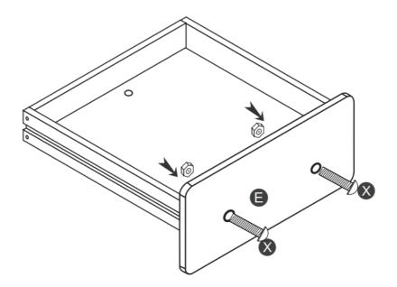
Align the assembled drawer with the sliding track inside the rail table and install the T cart (as shown in the diagram).
