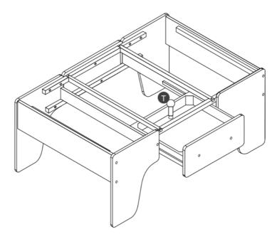
Place the R-Q-R components on the rail table and stick the Y stickers on the screw holes (as shown in the diagram) for a total of 14 holes.
