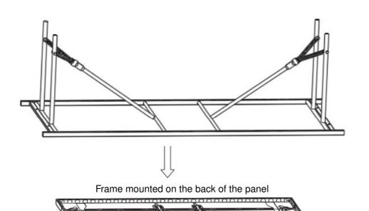
Don't tighten it until clamped into the feet tube (5)
