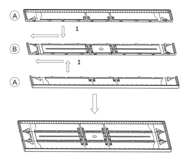
1. Align the card slot first, then push to the left to tighten it
