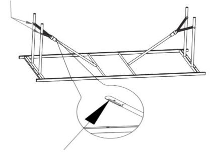
Note: This point is facing the direction of the panel frame while installing.
