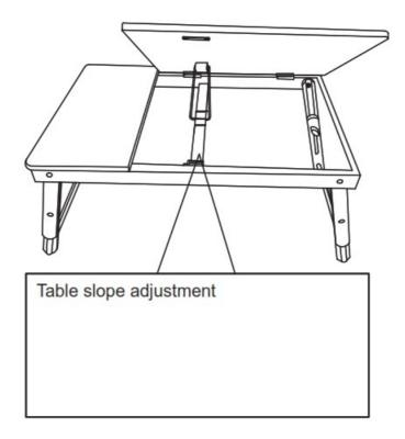
Adjust the table top to suit the slope (mark the position of adjusting gear) and complete the installation.
