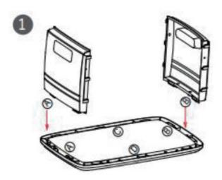
1. Find the bottom plate, the left (A), and right (B) side panels. Insert the left (A) and right (B) side panels into the corresponding slots on the bottom plate, as shown in Figure 1.
