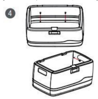
4. Reinforce the front and rear panels with two screws respectively, and then reinforce each of the four corner posts with a screw, as shown in Figure 4.
