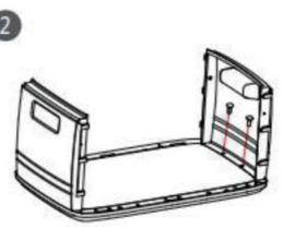
2. Reinforce left and right side panels with two screws on each side, as shown in Figure 2.
