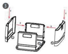
3. Insert the buckles of the front (D) and rear (C) panels into the side panels in the X direction and then insert them into corresponding slots on the bottom plate in the Y direction, as shown in Figure 3.
