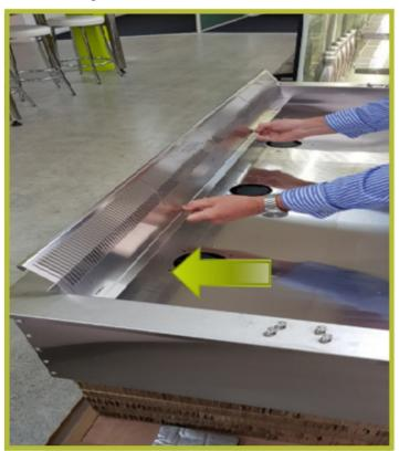
4. Lift panel to expose fans and coil
