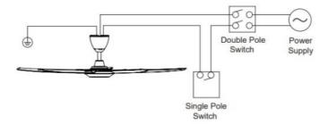
**IMPORTANT**: DO NOT CONNECT THIS REMOTE CONTROL CEILING FAN TO REGULATOR OR DIMMER SWITCH.
