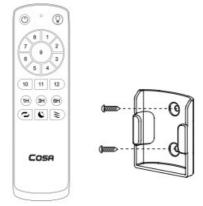
Mount the remote control holder on the wall with the screws provided.
