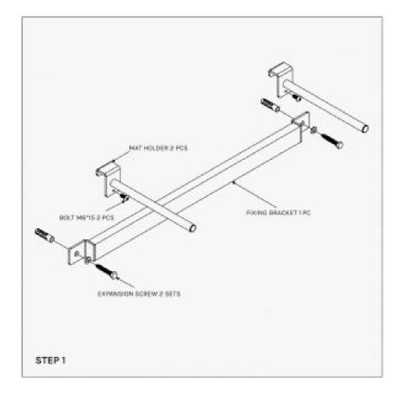
Install the mat holders as pictured below using the Bolt M6\*15 using a cross screwdriver.
