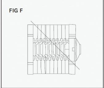
**STEP 5:** After use return BARBELL to base unit. Make sure that the Male/Female connectors are aligned. **STEP 6:** Make sure that the Male/Female connectors are aligned. Do not use if connectors are damaged.
