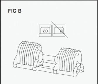
STEP 1: Place the BARBELL in the base unit. Female and Male connectors must be aligned.
