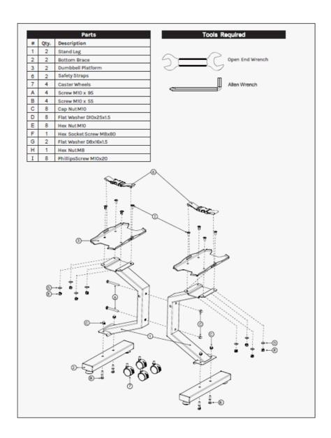
Connect 2x Screws M10 x 95 (A) and 2x Nuts M10 (C) to 2x Stand Leg (1).
