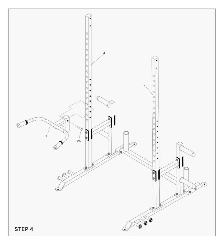
1. Plug the Dip Frame (9#) into the Tall Vertical Frame (4#). You can choose the left side or right side. Push the Ball Pin (25#) into the holes on Tall Vertical Frame (4#).
