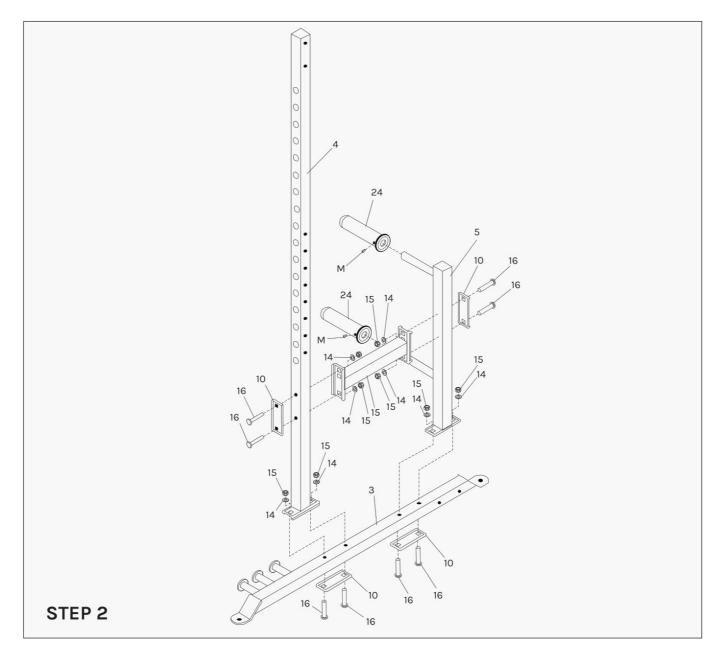
1. Attach the Tall Vertical Frame (4#) and Short Vertical Frame (5#) to the Left Base Frame (3#).
