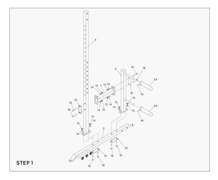
1. Attach the Tall Vertical Frame (4#) and Short Vertical Frame (5#) to the Right Base Frame (2#).
