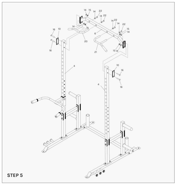
1. Attach the Lat Support (6#) to the left and right Tall Vertical Frame (4#).
