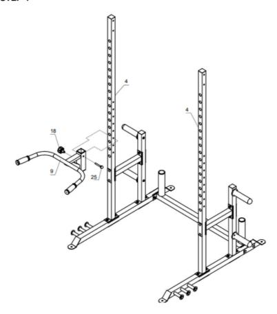
1. Plug the Dip Frame (9#) into the Tall Vertical Frame (4#). You can choose the left side or right side. Secure with Lock Knob (18#) and Push the Ball Pin (25#) into the holes on Tall Vertical Frame (4#).
