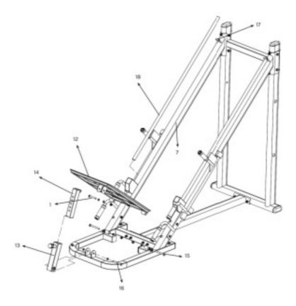
• Secure part #13 adjusting the intubation onto #9 using, #16 M10-90
