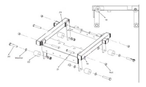
• Place #19 roller into #23 slide frame and use #21 M14-90 bolt (washer is not needed here) and tighten the nut.
