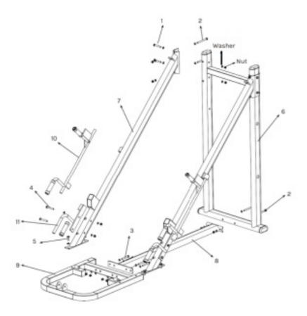
• Use part #3 M10-80 bolt, #2 M10-120, and #1 M10-70 to secure part #6 main frame, #8 bottom frame support and #9 foot pedal bracket together.
