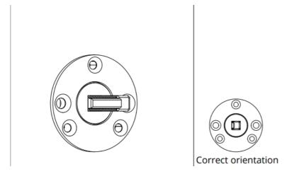
9. Screw the rose on to the fising plate and then the handle on to the spindle
