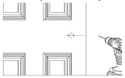
3. Drill pilot holes for the wood screws with the 2mm bit.
