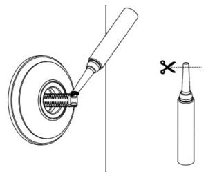
15. Replace the grub screw in the handle with the grub screws with pre-applied thread lock.
