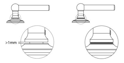
11. Screw the grubscrew in to the handle and make it it is level
