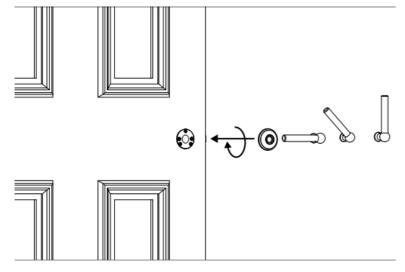
10. if after screwing the handle on there is a gap bigger than a 1mm between the handle and rose, use the washer to fill the gap.
