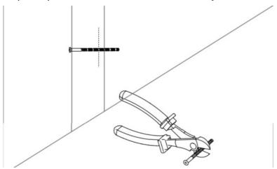
6. crew the fixed spindles to the door with the through bolts.
