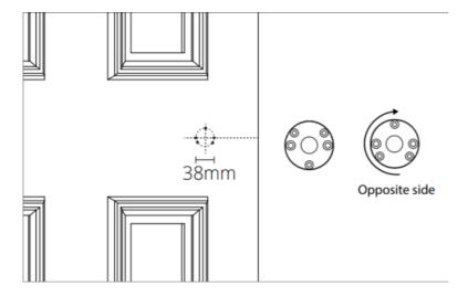
2. Drill holes through the door for the through bolts with the 8mm drill bit.
