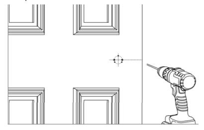
4. Using the 12mm drill bit, drill through the centre for the spindle.
