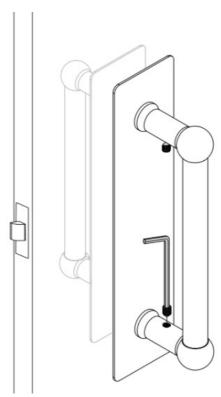
Using the 2.5mm allen key, tighten the four grub screws on the inside of the handle.
