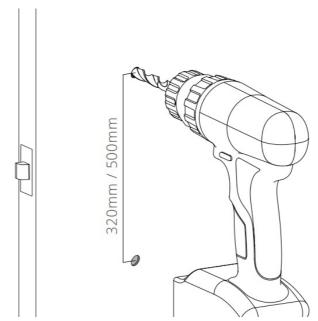
Mark and drill two holes in the timber door using a 10mm drill bit. Masking tape can be used to mark accurate holes and adjust positioning.
