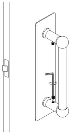
Using the 2.5mm allen key, tighten the two grub screws on the inside of the handle.
