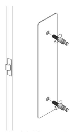
Screw anchors into door over plate and tighten by hand. Use a spanner for more robust doors.
