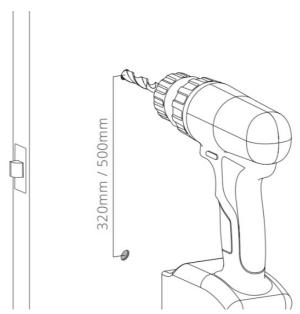
Mark and drill two holes in the timber door using a 10mm drill bit. Masking tape can be used to mark accurate holes and adjust positioning.
