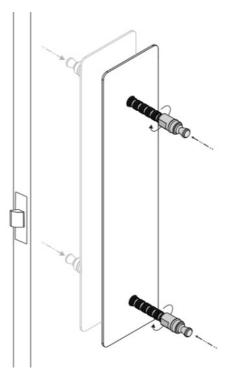
Screw anchors into door over plate and tighten by hand. Use a spanner for more robust doors.
