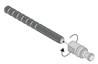
Insert threaded bar all the way into handle anchor.
