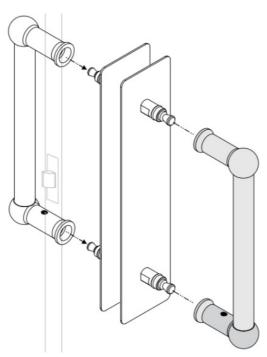
The handle can be attached to the anchors. Both ends of the handle should be flush to the plate or the door
