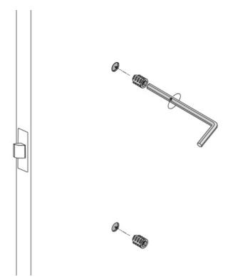
Use an 8mm allen key (not provided) to drive the insert nuts into the holes. Ensure the insert nut is flush with surface.
