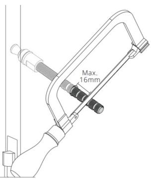
Insert the threaded bar though the door and mark 16mm of thread through the other side. Cut the threaded bar on a thread clearance with a hacksaw.
