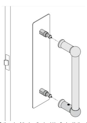
Attach handle to the anchors. Both ends of the handle should be flush with the plate/door
