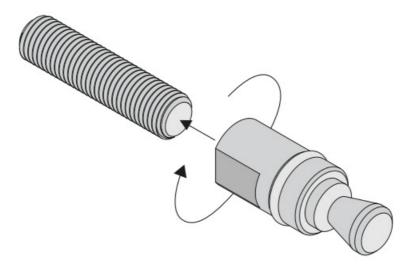
Insert threaded bar all the way into handle anchor.
