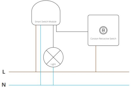
Example wiring\* (wiring varies between modules)
