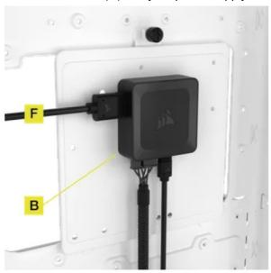
Mount iCUE LINK System Hub to your case. The iCUE LINK System Hub (B) can be magnetically mounted on a steel chassis or adhered to a surface with the supplied mounting tape.
