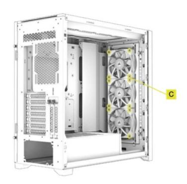
Mount the RX RGB fans onto your casewith the supplied uikTurn mounting screws (C). Please note that uikTurn screws thread much faster than traditional self-tapping screws; we advise hand-tightening uikTurn screws with a screwdriver only to avoid over-threading your RX RGB fans.
