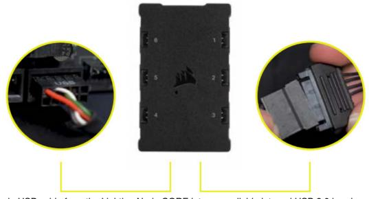
Plug the 9-pin USB cable from the Lighting Node CORE into an available internal USB 2.0 header on your motherboard or USB hub.
