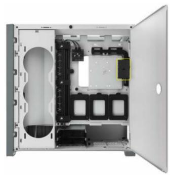
Find a location for the Lighting Node CORE that allows the fan RGB LED cables to reach the Lighting Node CORE, then mount it with the provided mounting strips.
