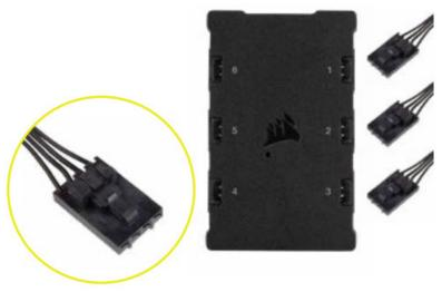
Connect the 4-pin RGB connectors from your AF120 RGB SLIM fans into the Lighting Node CORE controller in sequential order from port #1 to #6.
