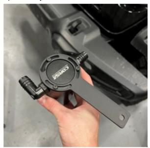
2. Using a 10mm socket, remove the bolt located next to the brake fluid reservoir on the driver's side. Install the catch can bracket using factory bolt to secure the catch can. Make sure the 90 degree fitting is installed in port B and straight fitting in port A of the can to properly route hose.
