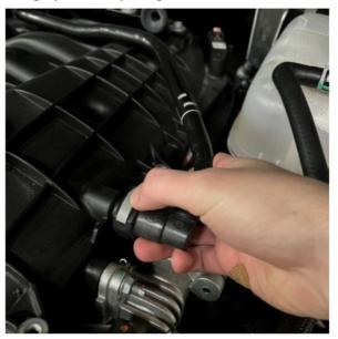
3. Locate and remove the opposite end of the PCV line attached to the crankcase on the back corner passenger side of the engine bay.
