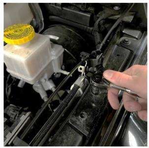
3. Attach quick disconnect fittings to 1 end of each hose. Attach Hose A to the crankcase side of the PCV system. Route the house back along the firewall and underneath the coolant reservoir and attach it to port A of the Catch can.
