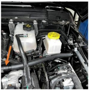
5. Make sure all fittings are secured in place and hose is pushed all the way over the barbed ends of the fittings.
