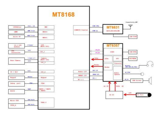
Processor: MediaTek MT8168, Quad-core ARM® 2.0GHz Cortex-A53 MPCore
