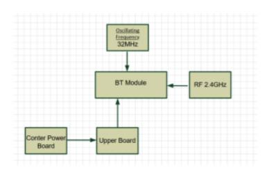
The Conter Power Board provides power to the Upper Board, which supplies power to the BT Module
