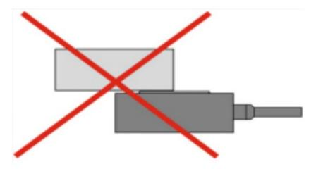
Excessive length of screws selected in the fastening and connecting process will lead to failure in installation or leakage of bolts, which will expose the product and scratch the product, affecting the motion accuracy of the product. Short bolts will lead to insufficient compactness of the connection and easy looseness, which will damage the internal structure of the product during operation.
