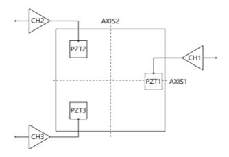
Assume that the max. control voltage is A, The control mode is as follows:
