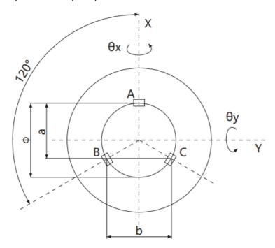
S23 has build-in three piezo actuators connected in parallel to provide the top ring motion. For vertical positioning (piston movement), it requires a controller with only one drive channel and three drive channels when it is in Z-direction and tip/tilt motion.
