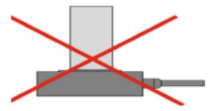
It is forbidden to load the load on one side of the piezo stage, which would cause serious damage to the product, as shown in the following figure:
