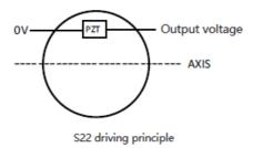
The piezo tip/tilt mirror is designed based on a single piezoelectric ceramic structure, using piezoelectric ceramic, deflecting movement in a push-pull mode stroke, and using a bridge connection circuit control, which could eliminate the influence of temperature on the piezoelectric ceramic, under a wide range of temperature changes Maintain good angular stability.
