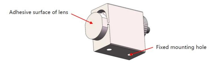
1. Clean the flat surface of the lens before pasting the lens, wait for a period of time after the lens is pasted, and then install it fixedly;
